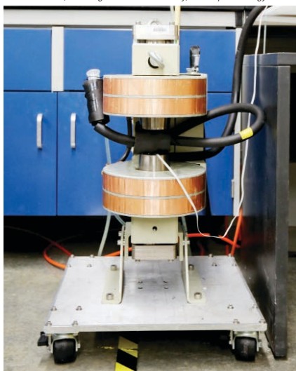
FIGURE 2. The magnetocaloric refrigeration system being developed at ORNL uses a magnetic field to remove heat
